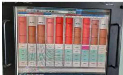
Gambar 2. Cargo oil tank display pada cargo monitoring system
