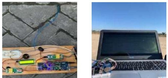
Gambar 9. Uji coba Transceiver LoRa dan Receiver LoRa
