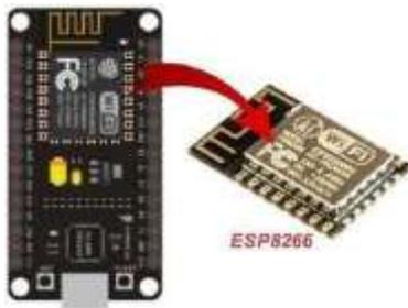
**Gambar 4.8** NodeMCU V3 ESP8266
