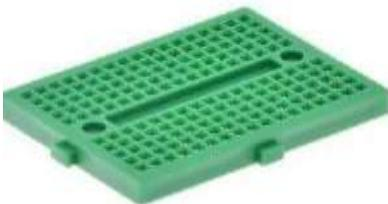
**Gambar 4.9** Mini Breadboard
