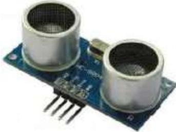
Gambar 1. Sensor Ultrasonik
